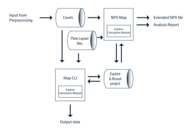
NPX Map is a command-line interface (cli). The application is capable of performing normalization, Quality Control (QC) and CV computations on NGS data, and exporting the results on several supported formats.
