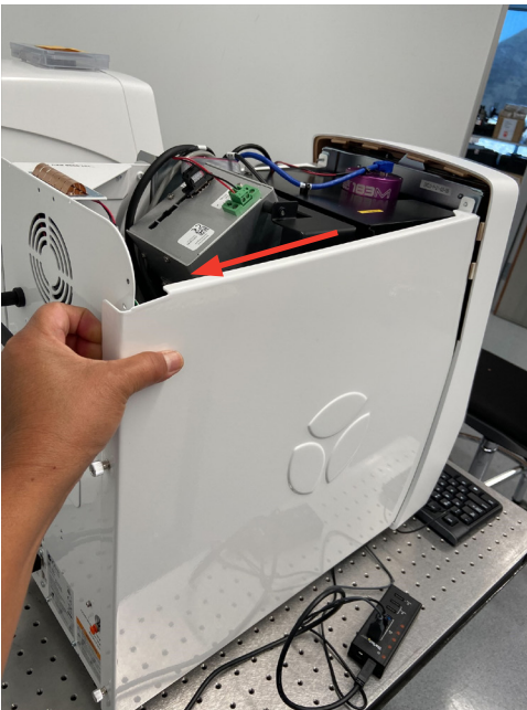
Figure 14. Removal of the left side panel
