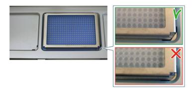
IMPORTANT: Risk of instrument damage! If the magnetic clamp booster is not correctly placed it may collide with the internal parts of the instrument during the run.
