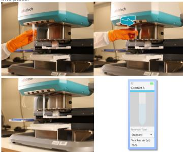
**NOTE:** Successful insertion of the syringe is indicated by a green symbol at the corresponding syringe position in the Setup page.
