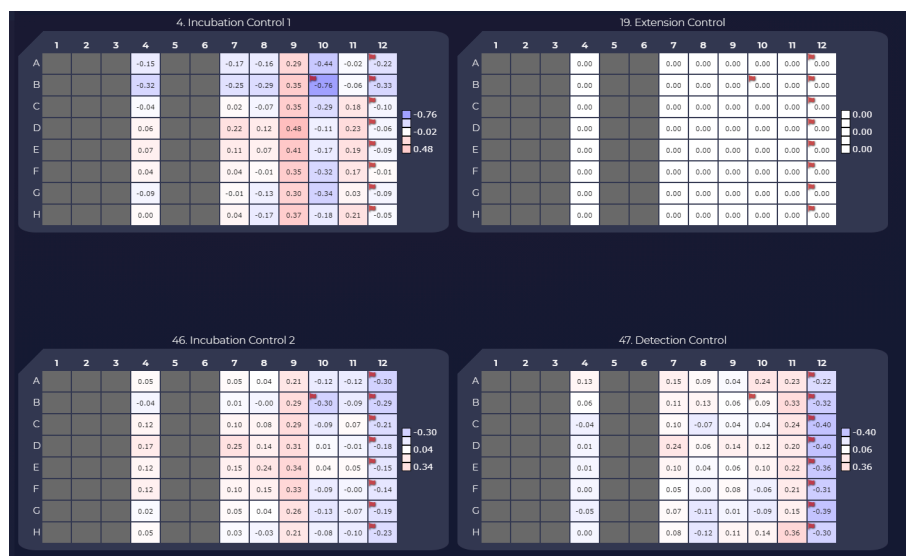
Figure 8. NPX values that show results of laboratory mistakes. Refer to table below for description of errors performed on this run.
