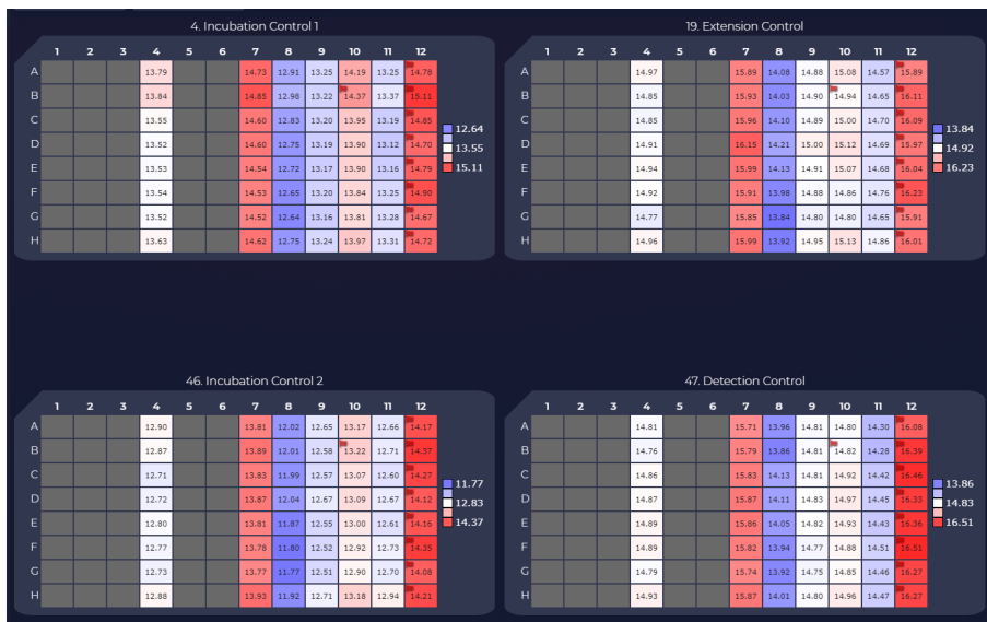
Figure 7. Ct-values that show results of laboratory mistakes. Refer to table below for a description of errors performed on this run.
